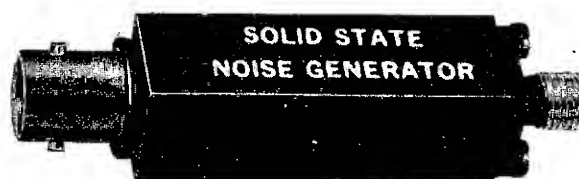
d) 07660 Typical High Level System Noise Source
